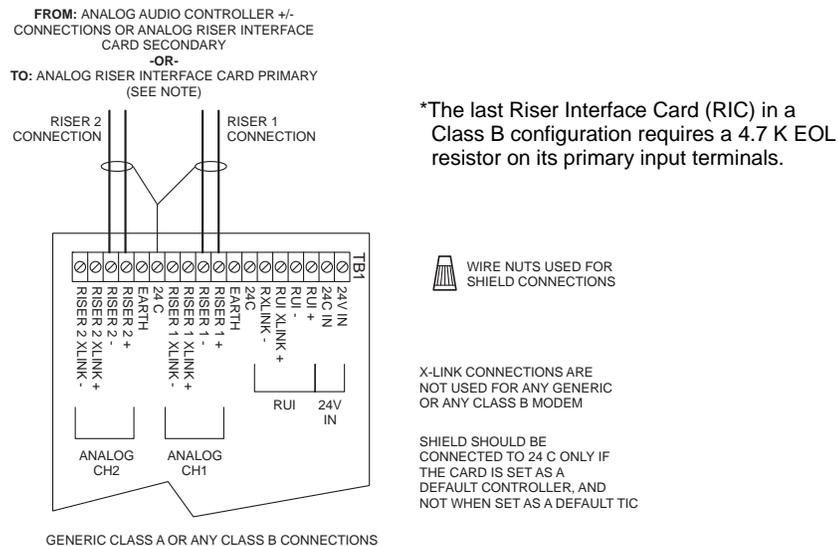
**Figure 8. Modem to Analog Audio Riser Wiring Diagram**
