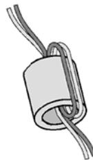
**Figure 6. Loop wires through bead as shown**
