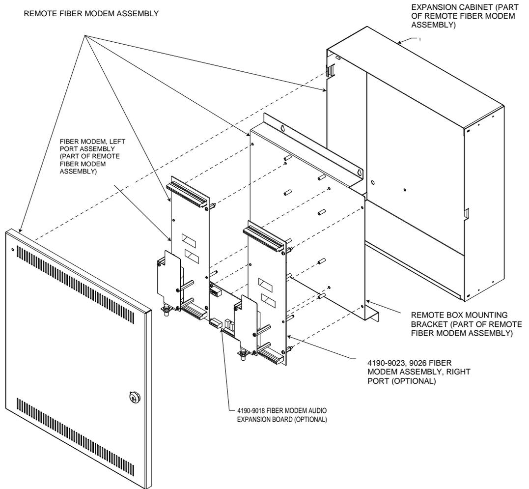
**Figure 4. Modem and Audio Expansion Board Mounting in a 4190 Remote Expansion Cabinet**
