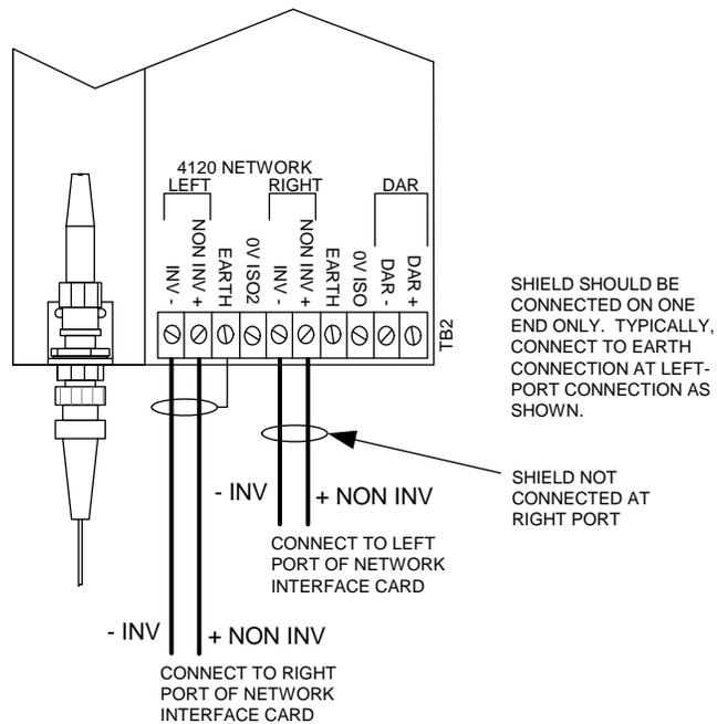
Figure 7. Modem to 4120 Network Wiring Diagram
