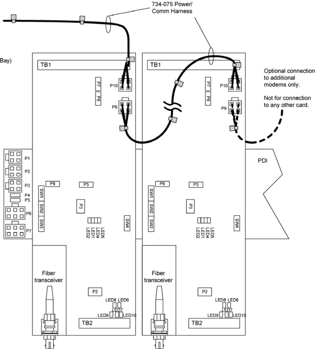
Figure 14. Modem Power Connections
