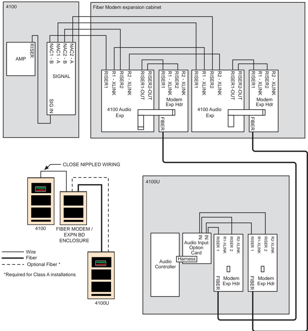
Figure A-21. Fiber Modem Audio Expansion Board, Class A/Style 6 (4100U Shown)
